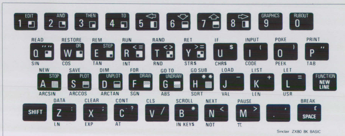
Keyboard template for new 8K BASIC ROM.
